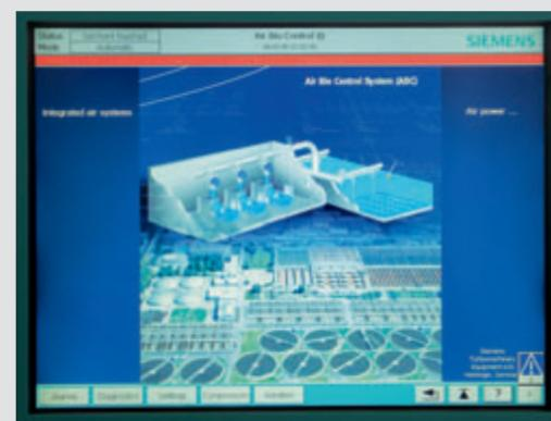
Based on a mathematical model of optimum aerobic conditions for the bacteria used in biological wastewater treatment, Siemens' Air-Biological Control (ABC) provides for a further boost in energy savings by adding a new level of accuracy to the aeration control system.
