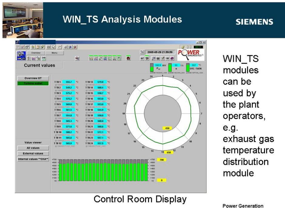
**Figure 3:** WIN\_TS™ screen for direct online monitoring at the plant.
