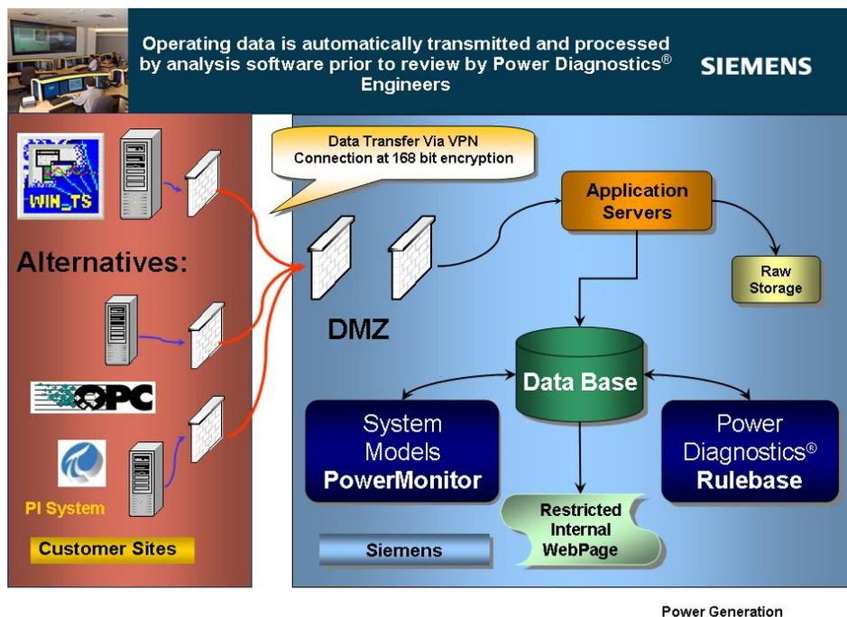
**Figure 2:** Data acquisition, transfer, and processing/evaluation/storage in the Power Diagnostics<sup>®</sup> Centers. Before the incoming data can enter the PDC, they are checked in the Demilitarized Zone (DMZ), a data storage area protected by firewalls.
