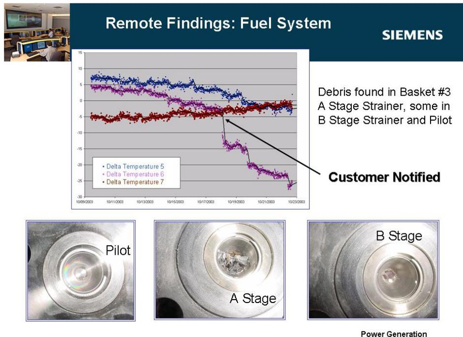
**Figure 7:** Debris in the fuel nozzles of a gas turbine, predicted and actually found after opening the engine.
