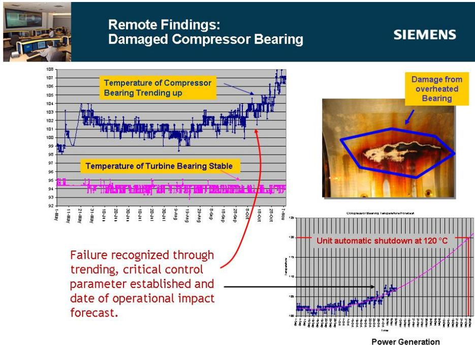
**Figure 8:** Early detection of a bearing issue by remote monitoring well before the I&C system would have alarmed. By counter measures the unit could be operated until a scheduled outage.
