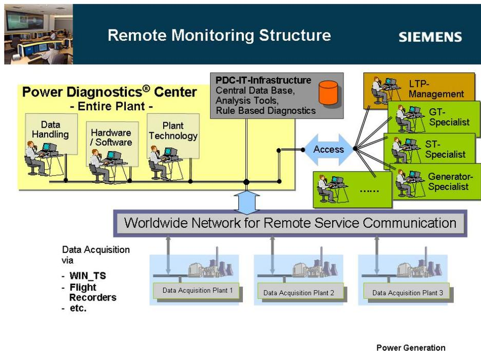
**Figure 1: Power Diagnostics<sup>®</sup> Remote Monitoring Infrastructure**
