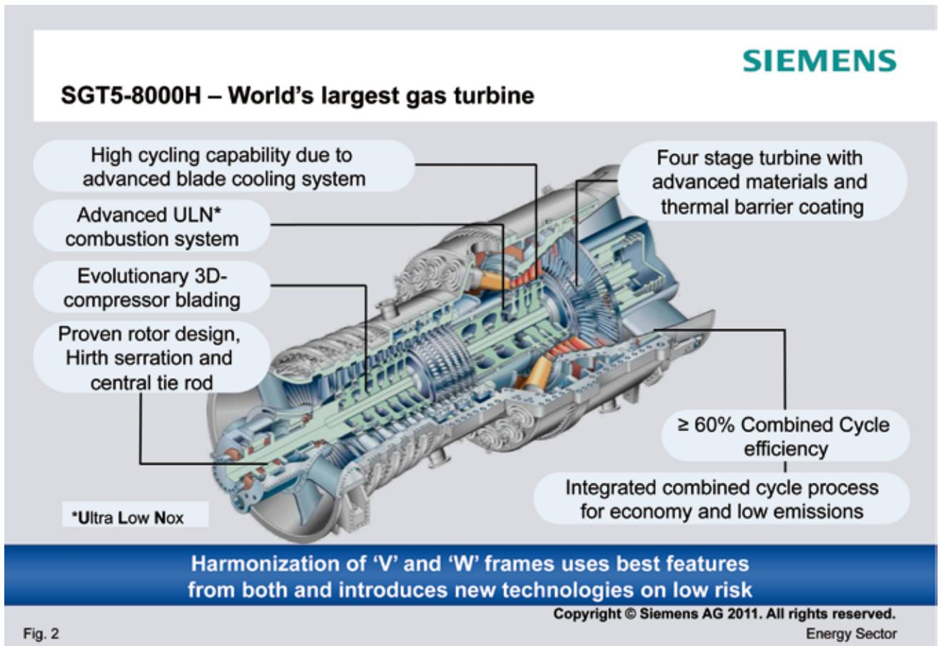
The air-cooled 8000H-technology gas turbine is a 1500°C-class design with 800 kg/sec inlet mass flow and 625°C exhaust gas temperature (Fig. 2).
