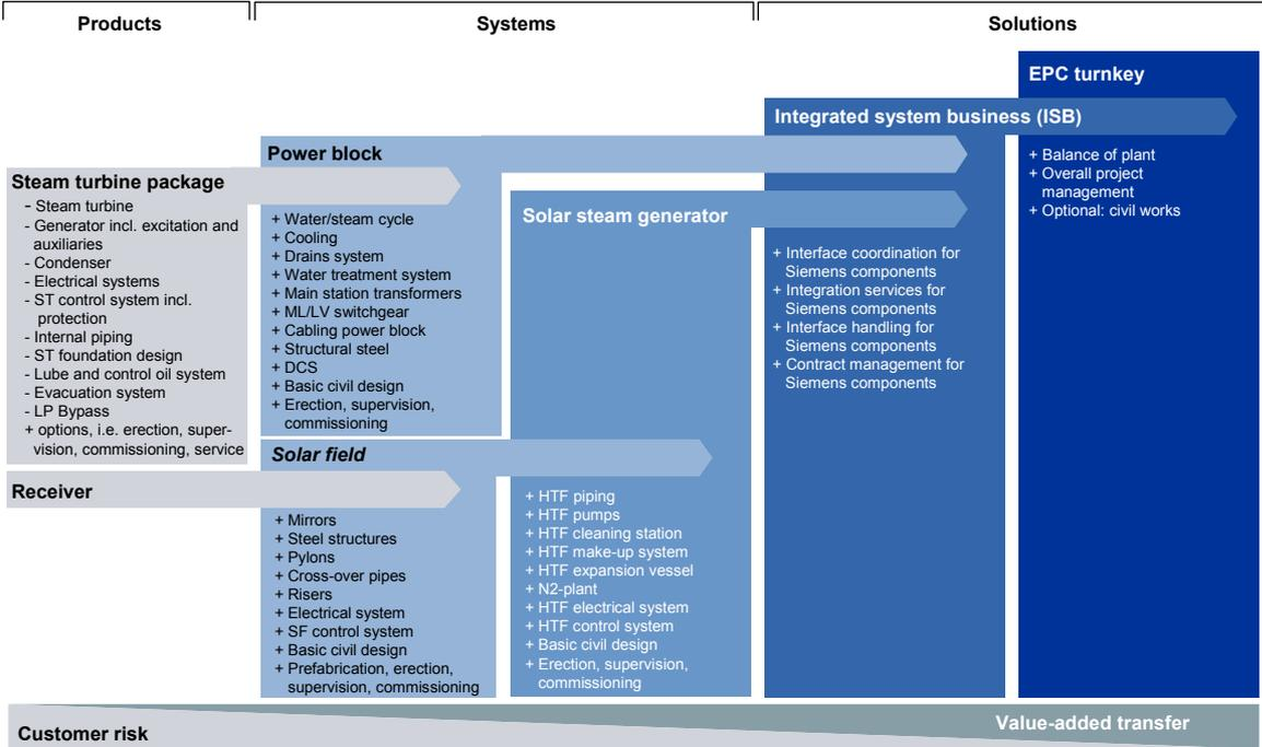
Figure 2: Products and systems of a concentrated solar power plant
