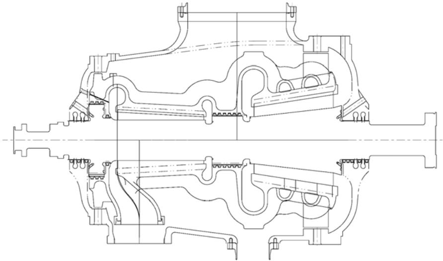
Figure 6: Longitudinal cross section of HI turbine for CSP application
