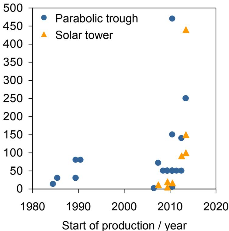
Figure 1: Production start vs. net power of parabolic trough and solar tower plants [3]
