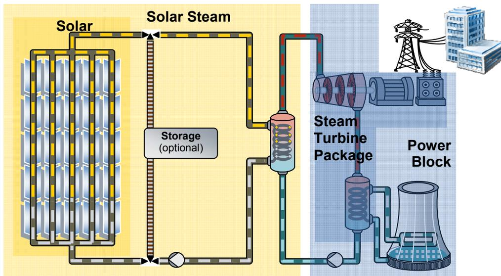
Figure 3: Main components of a CSP plant
