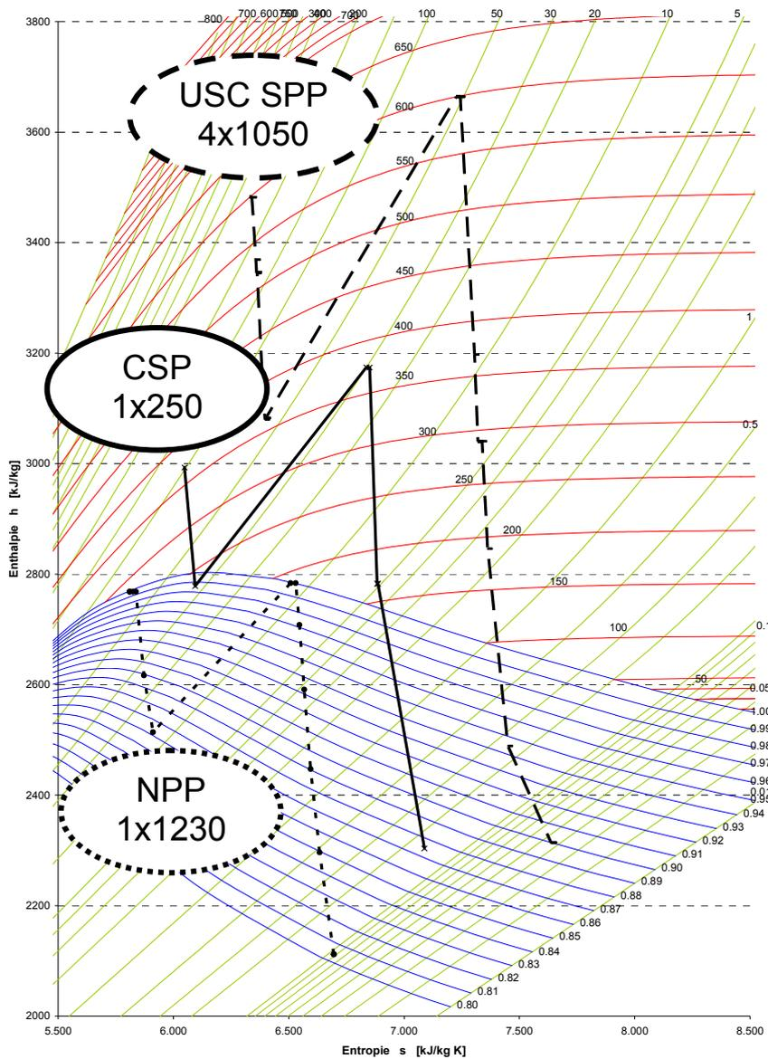
Figure 4: h,s diagrams of different typical steam cycles for Siemens large scale steam turbine applications
